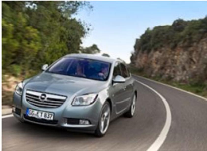
The Opel Insignia is now also available with a 1.4 turbocharged LPG ecoFLEX engine designed to run on liquefied petroleum gas (LPG). All three body styles of the award-winning Opel flagship - the sedan, hatchback and Sports Tourer station wagon - can now be ordered with LPG propulsion ex works. The new Insignia LPG ecoFLEX variant achieves an output of 103 kW/140 hp, only uses 7.6 liters on 100 km.
